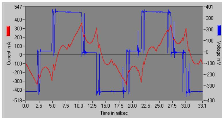
shows the voltage that a VFD, running at almost a 6-pulse mode, will send to the motor. The distorted currents are the motors reaction to the poor power condition. Very severe distortions are evident. This scenario shows a NEMA derating of 0.7. This allows the motor to be operated at 70% output.
